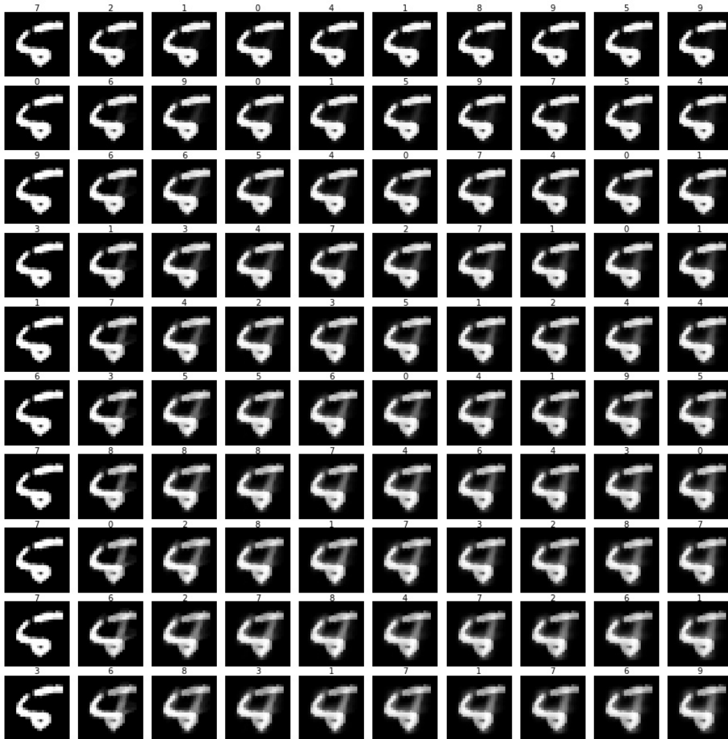
Figure 6: Generated adversarial example of Convolutional Neural Network as we increase the distance d (1 to 10) and perturbation magnitude \epsilon (0.1 to 1.0) with a uniform pixels \beta = 5 . Values above each image are the predicted class labels. The correct class label is 5 as predicted by CNN before applying an image perturbation.
