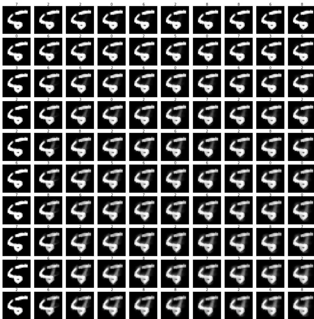
Figure 5: Generated adversarial example of Vanilla Neural Network as we increase the distance d (1 to 10) and perturbation magnitude \epsilon (0.1 to 1.0) with a uniform pixels \beta = 5 . Values above each image are the predicted class labels. The correct class label is 5 as predicted by VNN before applying an image perturbation.
